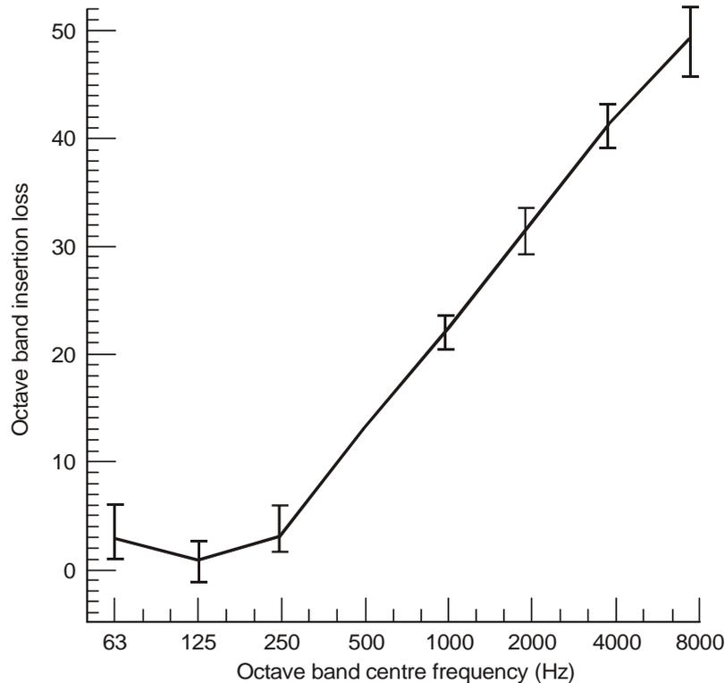
Figure 8.21 Typical pipe lagging insertion loss for 50 mm glass fibre, density 70-90 kg m<sup>-3</sup>, covered with a lead/aluminum jacket of 6 kg m<sup>-2</sup> surface density. The I symbols represent variations in measured values for three pipe diameters (75 mm, 150 mm and 360 mm).
